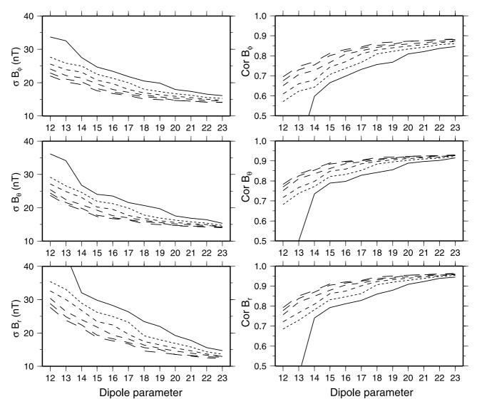
**Figure 2.** Left Panel: evolution of residual rms values with respect to the dipole parameter. Right panel: evolution of correlation coefficients with respect to the dipole parameter. From solid to long dashed line, depths = +10, 0, -10, -20, -30 and -40 km, respectively. From bottom to top,  $B_r$ ,  $B_\theta$ ,  $B_\varphi$ . Relative evolution of the residuals is 1.0%.
