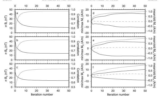
**Figure 1.** Statistics of the M22/-10 model series. Left Panel: evolution of rms (black line: left axis) and correlation coefficient (gray line: right axis) between observed and predicted values for a)  $B_r$ , b)  $B_{\theta}$  and c)  $B_{\phi}$ . Right Panel: minimum and maximum (black solid line: left axis), arithmetic mean (gray dashed line: right axis) and std mean magnetizations (gray solid line: right axis) for d)  $M_r$ , e)  $M_{\theta}$  and f)  $M_{\phi}$ .
