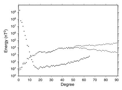
**Figure 5.** Energy spectra of the Earth's magnetic field from *Sabaka et al.* [2002] model (stars), and of Mars' magnetic field from our model (black diamonds) and from *Cain et al.* [2003] model (crosses).
